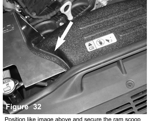
Figure 32 Position like image above and secure the ram scoop using plastic clips from step11.
