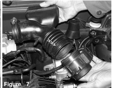
Figure 7 Loosen clamp that secures the air duct over the mass air flow sensor. Disconnect and remove the mass air flow sensor from the air duct as shown above.
