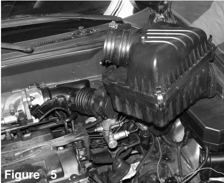
Figure 5 Disconnect air box cleaner from the air intake duct and lift the air box out of the engine compartment.
