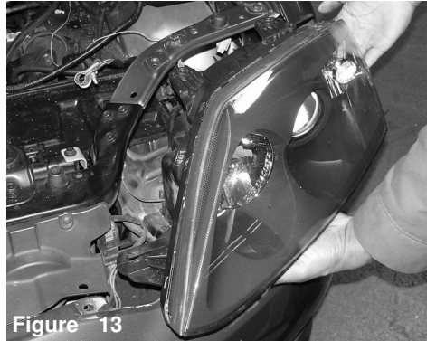
Figure 13 The head lamp is now pulled out of the frame and the harness clip is disconnected from the rear of the head lamp.
