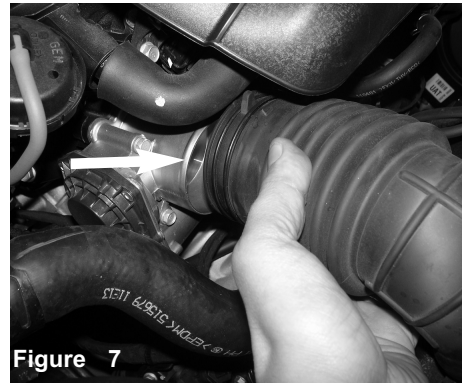
Now carefully pull back the intake hose from the throttle body.
