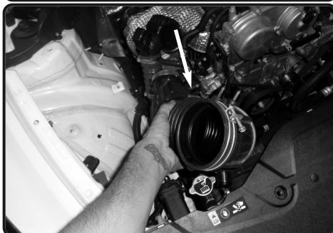
9. Remove the intake tube from vehicle.
