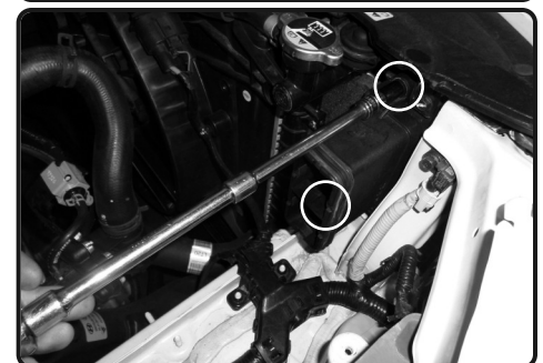
11. Loosen the 2 bolts holding in the front plastic ram unit and remove. Save bolts for later install.
