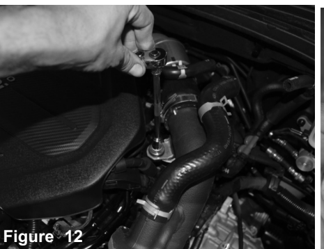
Figure 12 Loosen the bolt holding in the upper intercooler pipe to engine.
