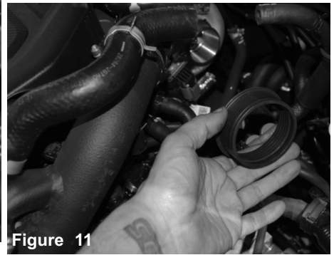
Figure 11 Remove the rubber coupler from the turbo.
