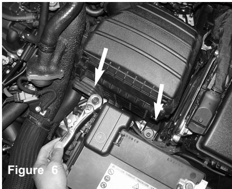
Figure 6 Use a 10mm socket/ratchet and remove the two M6 bolts in front of the air box assembly
