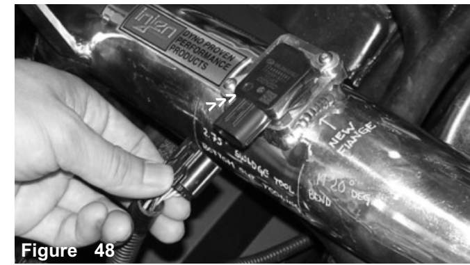
Figure 45 The mass air flow sensor is carefully inserted into the machined sensor flange. Use a dab of light oil around the O-ring to prevent it from kinking or tearing.
