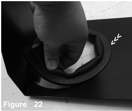
Figure 19 The stock vibra-mount is also removed from the bracket on the fender wall.
