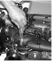
Figure 6 The electrical harness clip is disconnected from the mass air flow sensor.
