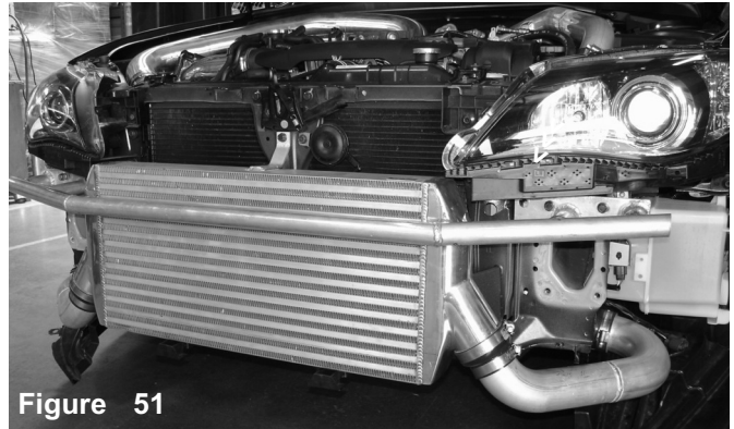
Figure 51 Coming soon, the SES1204FMGT- Large front mount intercooler with a replacement bumper support and intercooler piping.
