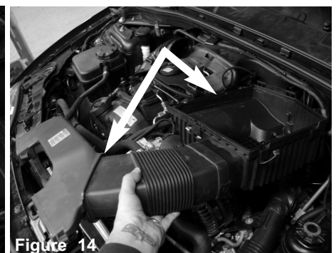
Figure 14 Lift and pull up the lower air box assembly from the 3 grommets attached to the engine and remove.
