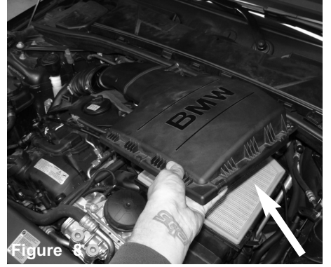
Figure 8 Lift and remove the upper half of air box out of vehicle.
