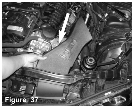
Figure 37 Install the driver side factory scoop, position the injen power-scoop to the back of the core support, locate the 2 inserts through the scoop. Secure the power-scoop using the 2 remaining M6 button head screws.
