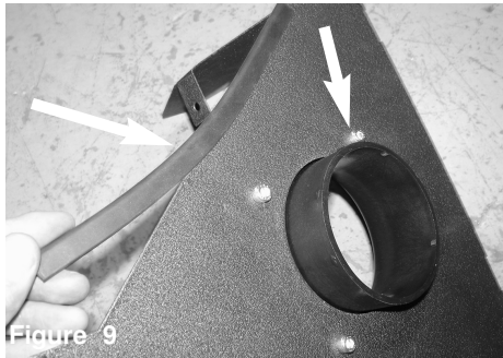
Figure 9 Secure the Velocity stack adaptor using provided m6 allen screws. Install the vinyl trim to the edge of the heatshield.
