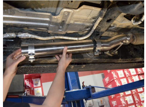
6. FOUR DOOR MODELS ONLY: Attach the mid pipe extension to the front pipe. Secure using the provided 76mm clamps.
