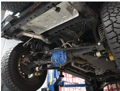
11. If needed loosen all clamps and adjust fitment of the exhaust. Once finished secure all bolts and clamps.
