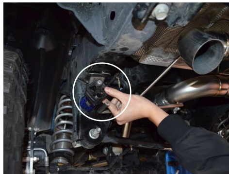
8. Insert the driver side hanger into the rubber insulator.
