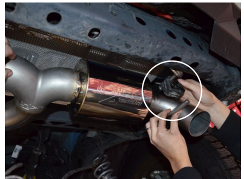
9. Insert the passenger side hanger into the rubber insulator.
