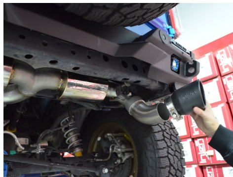
11. OPTIONAL: Attach exhaust tips to the tip extension.
