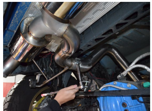
12. If necessary loosen the factory clamp and adjust the fitment of the exhaust.
