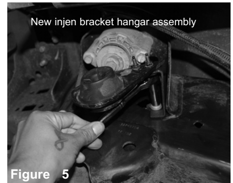
Figure 5 Secure and tighten the bracket using OEM M8 bolts from figure 2. Make sure the bracket is secured and tighten.
