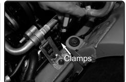
**31.** Secure and tighten clamps using 8mm nut driver. Re-install guard, and intake system. Your intercooler pipe kit is now complete.
