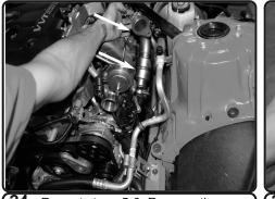
**24.** Repeat steps 5-6. Remove the driver side intercooler out of vehcile sliding behind the turbo out. This may require to maneuver piping.
