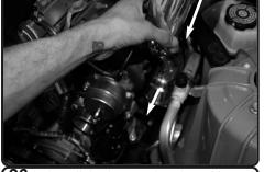
**26.** Install the intercooler pipe with machined fitting side first into same position, This may require to maneuver piping.
