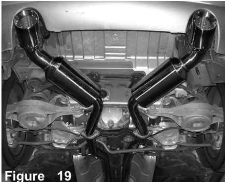
Figure 19 The rear mufflers are now installed. Make your final adjustments for best fitment and then tighten all M10 bolts
