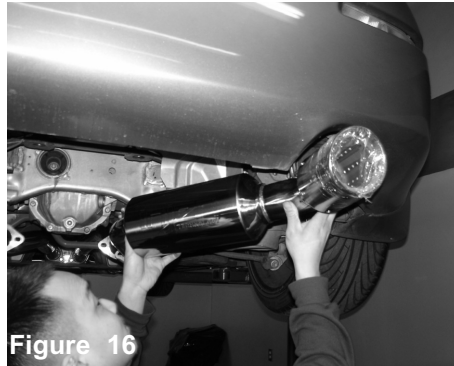
Figure 16 Place the rear right and left mufflers onto the hangers
