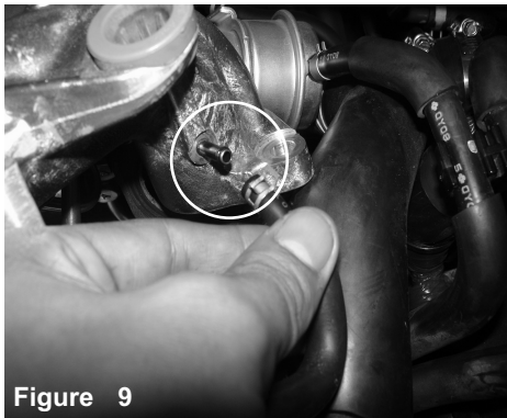
Figure 6 With 10mm socket and ratchet loosen the 2 screws holding in the vacuum valve.
