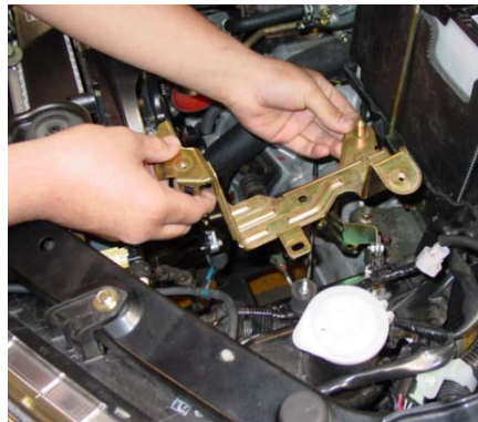
Remove the stock zinc plated brace that once held the air intake box and boost solenoid in place.
