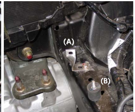
Take the small 1450T bracket and mount it to the frame of the car, use the stock bolt to secure the bracket in place(A). Screw the vibra-mount into the pre-tapped hole on the same frame as the bracket(B).
