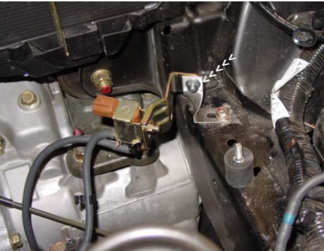
Mount the boost control solenoid bracket to the 1450T bracket. Use an m6 x m16 hex bolt and flange nut.
