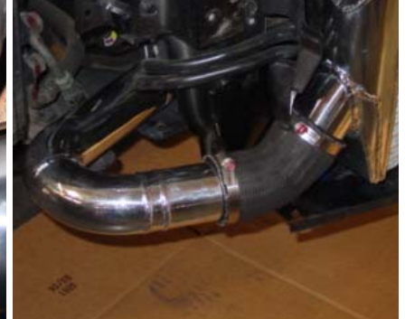
Here is a good shot of the 2 3/4" end inserted into the stock elbow located on the intercooler tank. Two .362 Power-Bands are used to secure the hard-pipes in place.
