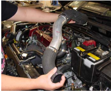
Remove the stock intercooler piping with the rubber with the stock hose connectors. The piping to the driver side front intercooler is removed with the exception to the connecting hose on the intercooler.
