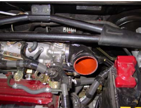
Press the 90 degree elbow on the throttle body and use two two .312 Power-Bands on the elbow. Semi-tighten the clamp on the throttle body at this time.
