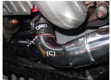
Hardpipe (C) connected to passenger side intercooler end tank inlet. The side seen here is the hardpipe connected to the turbo outlet.
