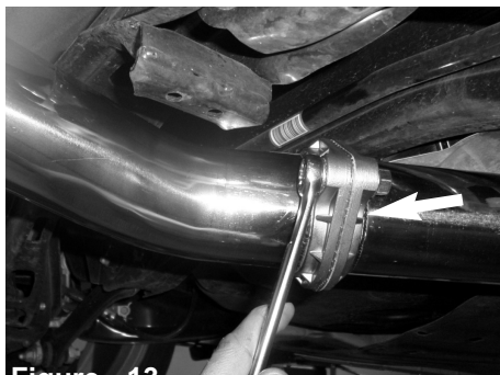
Figure 13 Position for best fit and clearance. Once the exhaust is in correct position, Secure and tighten. Secure the bracket assembly also. Note: Exhaust system has room for adjustment, re-position and tighten for best fit.
