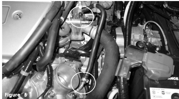
Coolant line (B) is reused to close the loop between the thermostat housing port and the throttle body port. Reuse the stock hose clamps to prevent any slipping.
