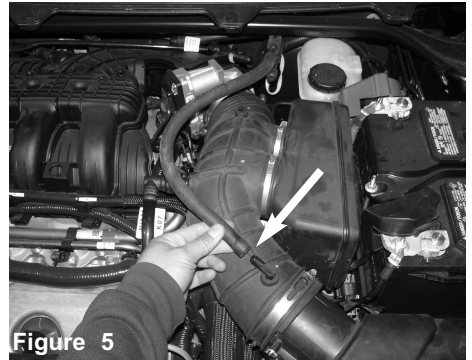
Detach the brake booster vacuum line from the top of the factory air duct
