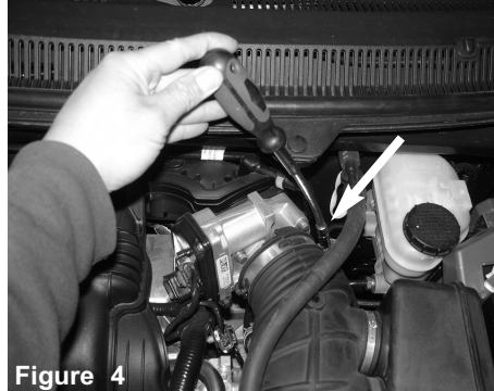
Use a 8mm nut driver and loosen the clamp on the factory air duct located on the throttle body
