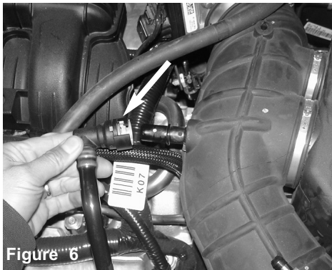
Pull the release tab on the left vacuum line located on the factory air duct to detach it from the fitting on the air duct
