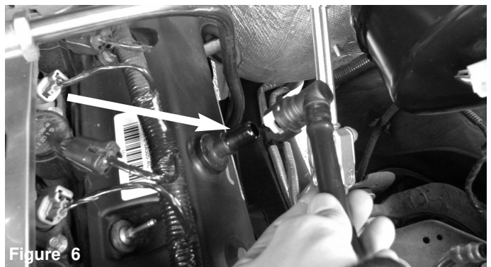
Figure 4 Loosen clamp on throttle body using 8mm nut driver.
