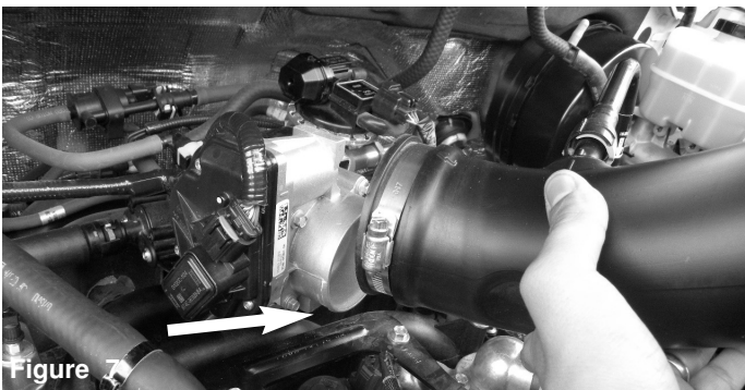
Figure 5 Disconnect MAF sensor harness.
