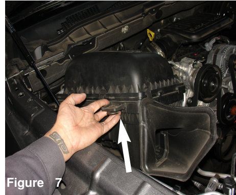
Figure 4 Loosen the clamp on the resonator box using 8mm nut driver.
