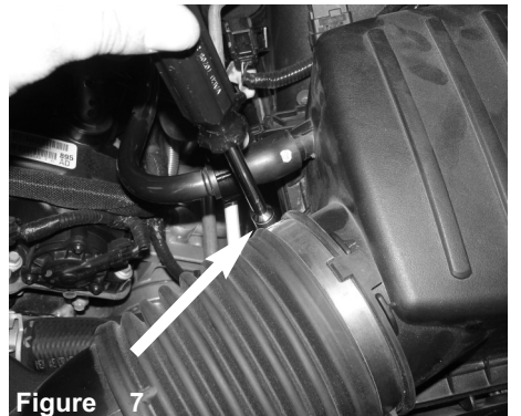
Figure 7 Loosen the clamp on the air box.
