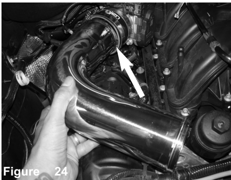
Figure 21 Install the 3-1/8" straight hose with clamps to the throttle body.
