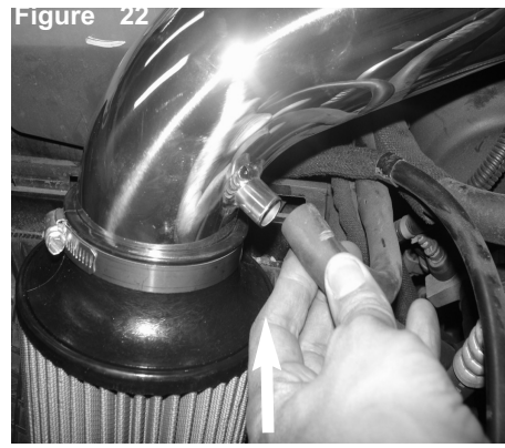
Connect the crank case line to the fitting on the intake tube.
