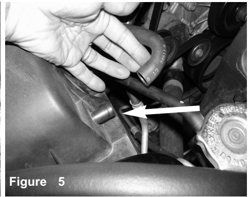
Figure 5 Pull back the crank case line from the air box.
