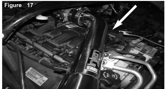
Figure 17 Install the intake tube into the vehicle and position to the throttle body and the bracket to the vibra mount.
