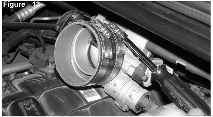
Figure 13 Tighten the clamp on the throttle body only.
