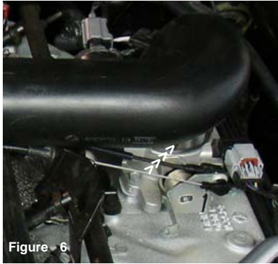
Figure 3 Remove the air temperature sensor from the air intake duct. (note: for Jeeps not equipped with air temp sensors, skip this step.)
