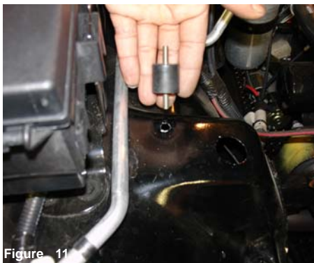
Figure 11 The vibra-mount is placed over the pre-drilled hole located on the fender well.
