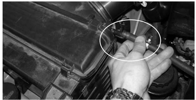
Disconnect the stock 8mm breather hose connected to the air intake box port. This line will be reused and connected to the first 1/2" port nearest to the filter.
