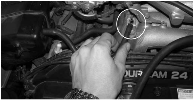
Disconnect the stock 6mm vacuum line connected to the small intake manifold port. This line will be replaced with the 27" 6mm vacuum hose.
