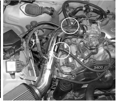
Congratulations! The intake is now install and the Injen vacuum lines have been installed.
