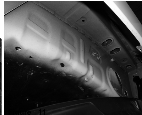
Figure 11 Under fender well compartment shown. This is where the filter will sit high tucked.
