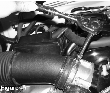
Figure 7 With 10mm socket and ratchet, loosen the clamp on throttle body.
