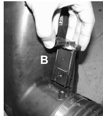
Figure 20 A) Install Maf sensor to new intake tube. B) Secure MAF sensor using M4 button head screws tighten using 2.5mm allen key.
