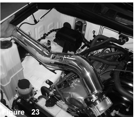
Figure 23 Install intake into vehicle and position.
