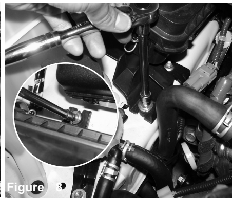
Figure 8 With 12mm socket and ratchet, loosen the 2 bolts holding in air box.
