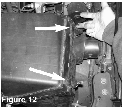
Figure 12 Unclip two retaining tabs holding the upper part of the air box to the lower part of the air box
