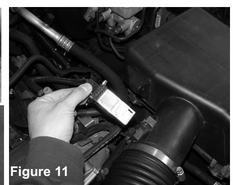
Figure 11 Now remove the MAF sensor out of the factory air box sensor housing. This MAF sensor will be reused later.
