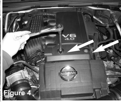
Figure 4 Use a 10mm socket with a 3/8 ratchet and remove the two 10mm bolts on the engine cover.
