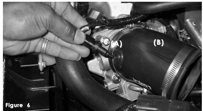
Figure 6 Press the sensor grommet in this kit into the hole in the elbow. Place the clamps over the beaded elbow and press the assembled elbow over the throttle body(B). Position the elbow in the correct direction and press the air temperature sensor into the sensor grommet (A).
