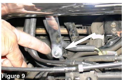
While the intake is pressed into the silicone elbow the bracket is lined up the the first vibra-mount stud, as shown above. Use the m6 flange nut and fender washer to bolt the intake bracket to the vibra mount.
