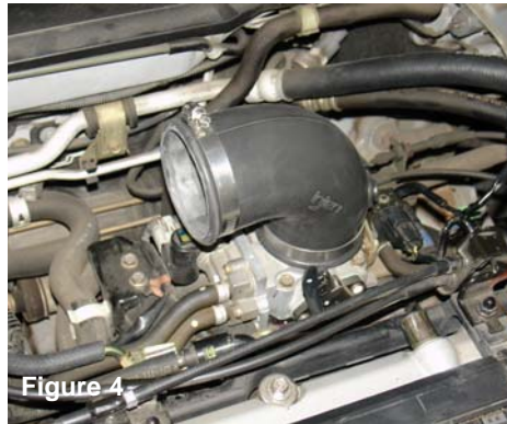
Place the one clamp on each end of the 90 degree elbow. Place the 90 degree elbow over the throttle body then semi-tighten the clamp on the throttle body.
