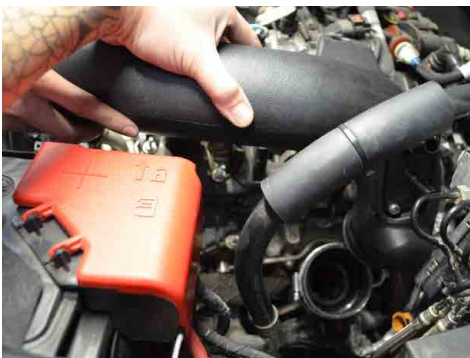
34. Insert the driver side tube into the 2.25"-3.00" Stepping hump hose. If needed remove the oil dipstick for clearance.
