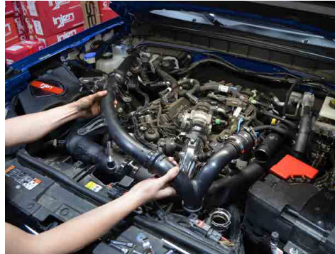
41. Reinstall the charge pipe.
