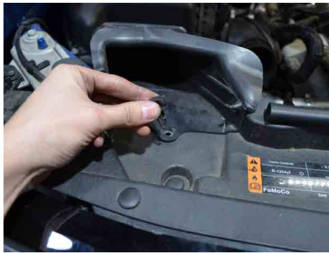
14. Remove the push clip securing the air box inlet to the front shroud.
