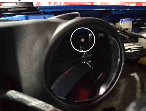
22. Install the airbox into the engine bay and secure the air box to the chassis with the factory bolt.
