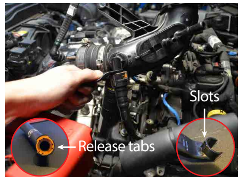
12. Line up the slots on the Injen release tool to the crank case fitting slots and firmly push up. This will unlock the tabs required to release the fitting.
