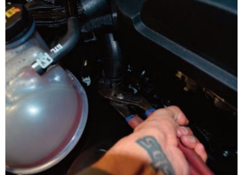
6. Squeeze the tension clamp until it locks into an open position. Then remove the BOV return line.
