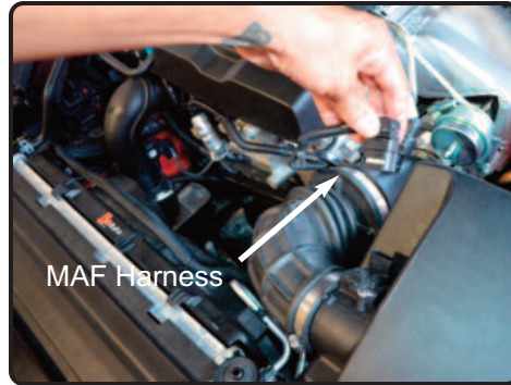
2. Disconnect the MAF sensor harness and pull line away from the intake tube.
