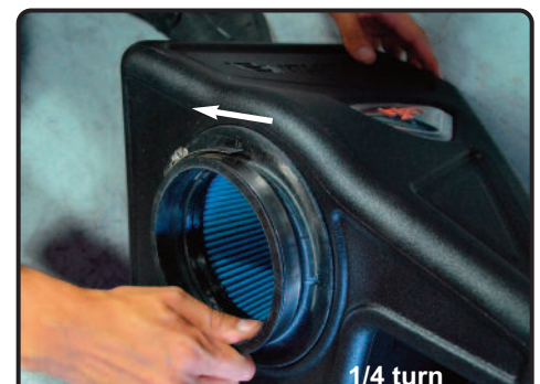
12. Now secure the Twist-Lock™ filter turning 1/4 turn in either direction. Make sure the filter locks into place.
