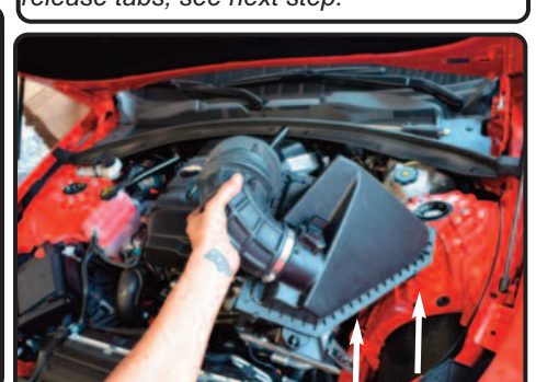
8. Now Lift up air box from vehicle and remove complete stock air box assembly.
