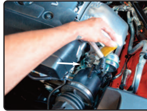
3. With 8mm nut driver, loosen the clamp on the throttle body and pull back tube from turbo.
