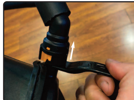
7. Line up the slots on the Injen release tool to the crank case fitting slots and firmly push up. This will unlock the tabs required to release the fitting
