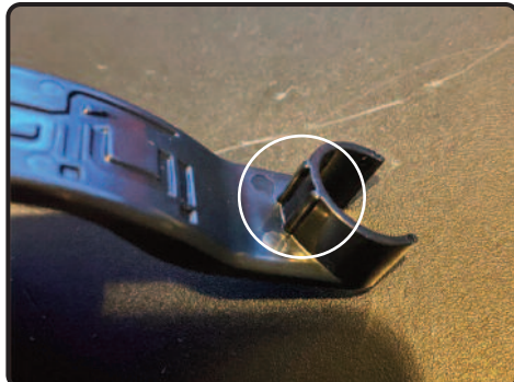
6. The supplied Injen release tool will have a set of slots that need to line up with a set of slots on the factory crank case fitting.
