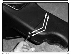
**16.** Secure the Injen scoop to the Injen air box using provided M6 button head screws and rubber washers. Secure and tighten using allen key.
