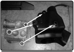
**11.** Remove the 3 grommet with crush-washer and install into the new airbox.
