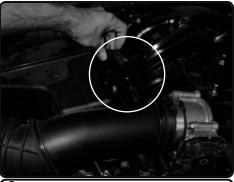
**3.** Now disconnect the Crank case fitting from the intake tube and pull back from tube.
