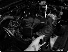
**5.** Now lift up and remove the stock intake tube from the vehicle.
