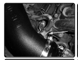
**24.** Reconnect the crank case line to the inien intake tube.
