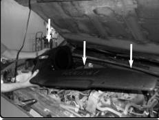
**17.** Install the air box assembly into the vehicle and position.
