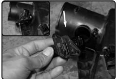
**8.** With phillips screwdriver, remove the two screws holding in the MAF sensor. Care-fully remove the MAF sensor.
