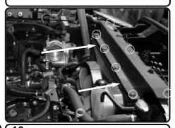
**10.** Loosen and remove the 7 push clips holding in the radiator plastic shroud and remove. Save 2 push clips for later install.
