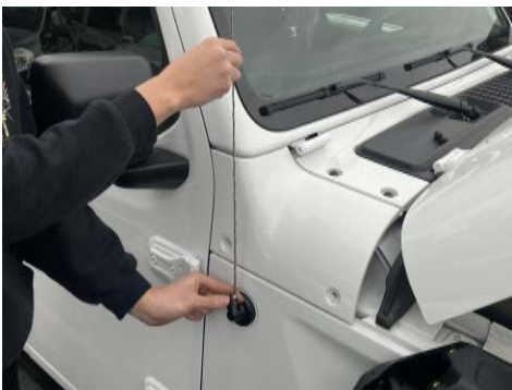
10. Remove the factory antenna.
