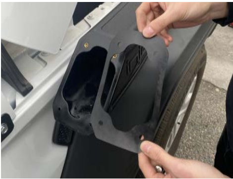
13. (OPTIONAL) Place the gasket on the lower snorkel. Refer to advisory on pg. 2
