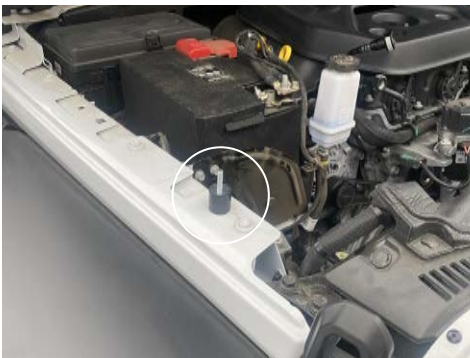
7. Attach the provided M6 vibra mount. The shorter end will be screwed into the chassis.
