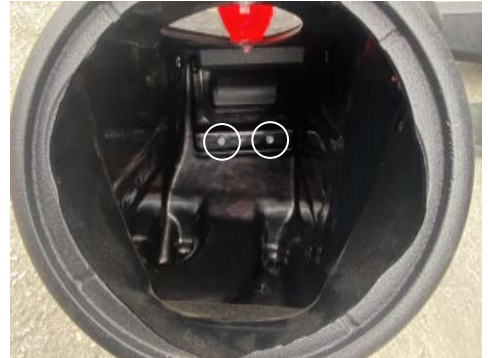
6. Secure the lower portion of the snorkel inlet to the air box with the provided M6 socket cap bolts.
