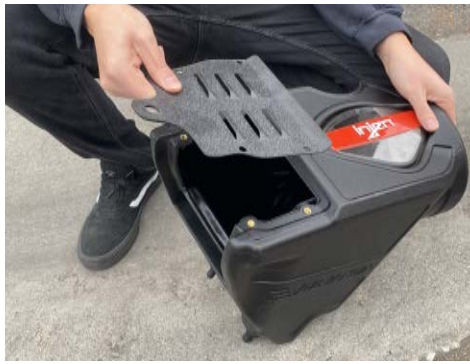
2. Remove the air box bracket.
