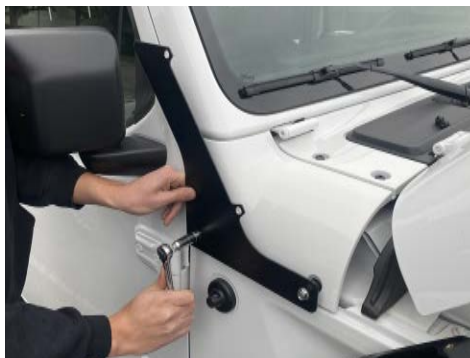
11. Bolt down the lower snorkel bracket using the two 40MM M8 bolts.
