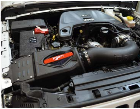
1. Remove the cold air intake.
