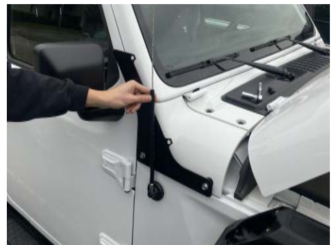
12. Slip the 6mm vacuum hose over the factory antenna then reinstall the antenna.
