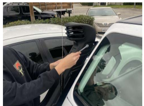
24. Bolt down the upper snorkel with the upper bracket using the two M6 x 1.0 x 16mm hex head bolts.
