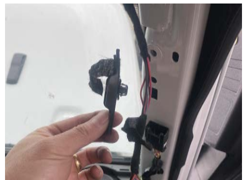
21. Remove the tape from the wire organizer clip attached to the harness. This clip will no longer be used.
