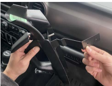
22. Line up the upper snorkel bracket with the top bolt on the pillar grab handle.
