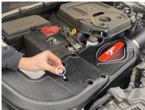
8. Reinstall the Injen intake and snorkel into the engine bay. Secure the snorkel to the vibra mount with the provided M6 nut
