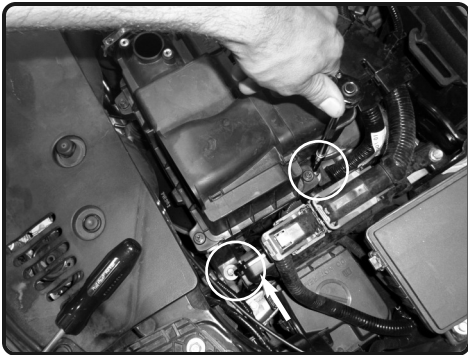
5. Loosen the 2 bolt holding in the airbox using 10mm socket and extension.
