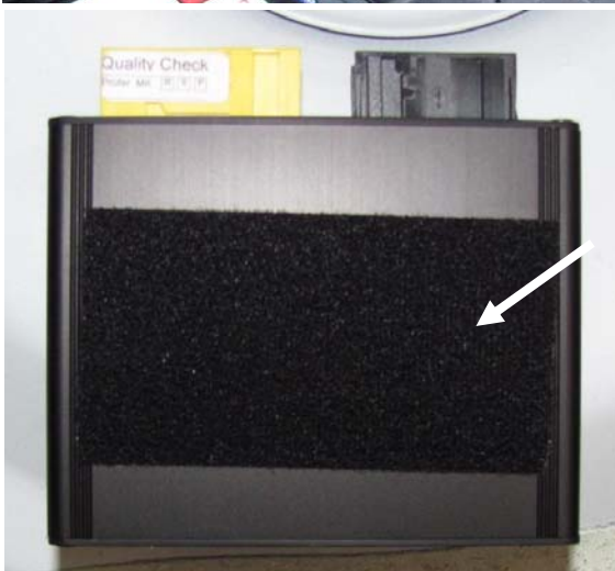
Klettband Hook-and-loop tape
