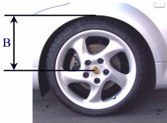
Measurement B Wheel hub center wheel arch
