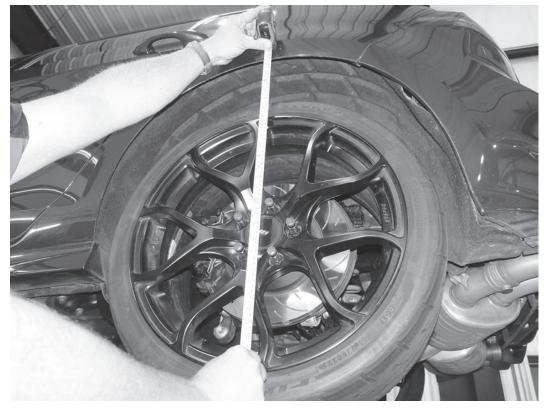
25) Measure the distance from the bottom of the rear fender to any vertical point down the center of the wheel, either to the top of the wheel, the middle of the wheel, or the bottom of the wheel. It only matters that you are consistent in what spot that you measure to on the wheel.
