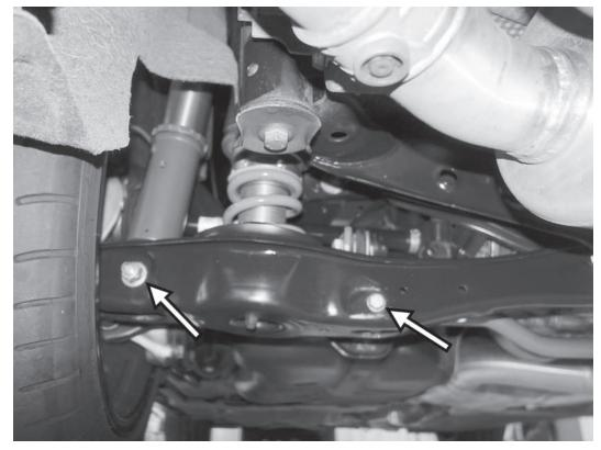
29) Loosely reinstall the lower shock bolt from the back of the control arm, and install the nut on the front side of the control arm. Once the other side has been done, reconnect the sway bar bolt from the back of the lower control arm. Leave all suspension bolts loose for now.
