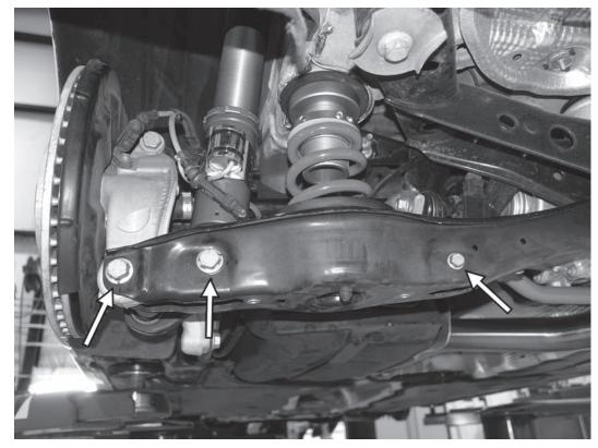
31) All suspension bolts should be tightened while the car is sitting at the set ride height. Tighten the bolt and nuts to the stabilizer bar lower link to control arm to 20Nm (15ft-lbs), and then tighten an additonal 90°. Tighten the bolt and nut holding the lower control arm to the rear upright to 70Nm (52ft-lbs), and then tighten an additional 180°. Tighten the bolt and nut holding the bottom of the shock to the lower control arm to 70Nm (52ft-lbs), and then tighten an additional 180°.
