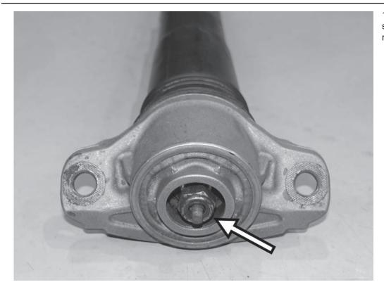
19) Remove the nut holding the rear shock to the upper shock mount, and remove the mount from the shock.
