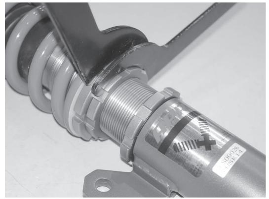
11) Adjust the preload on the spring. With the spring up against the bottom of the upper camber plate, hand thread the lower spring perch up to the bottom of the spring. Then, after measuring and with the supplied tools, tighten the lower spring collar an additional 10mm, preloading the spring on the strut assembly. Thread the upper locking collar against the lower spring perch, and then lock the two in place against each other.
