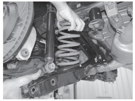
17) Pushing down on the lower control arm, remove the rear spring and the top factory rubber perches from the car. The lower rubber perch should stay attached to the lower control arm.
