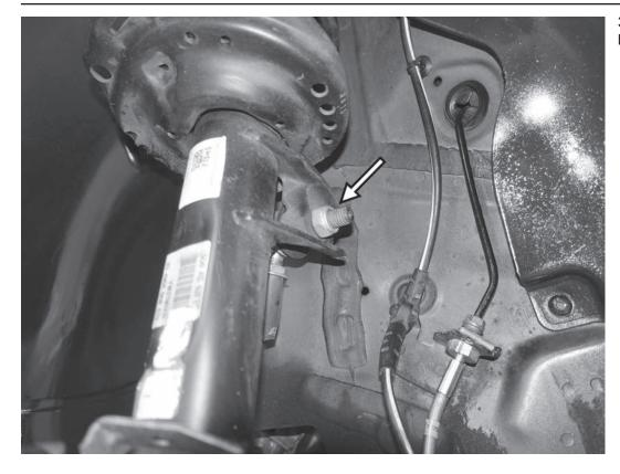
3) Disconnect the sway bar from the back of the strut body.
