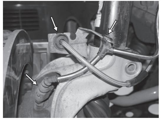
5) Disconnect the speed sensor harness from the speed sensor, and separate the harness from the bracket on the top of the upright. Separate the brake hose from the same bracket. If equipped, detach any ride height sensors to the upright, lower control arm, or the strut.
