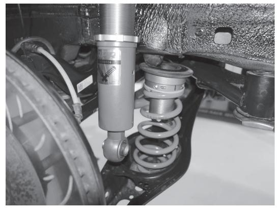
21) Install the rear spring assembly with the factory top rubber perch. The factory lower rubber perch should still be in the lower control arm. Note that the upper APR spring perch is threaded all the way up on the threaded body of the upper spring mount. This represents the lowest the car can go on the rear coilover.
