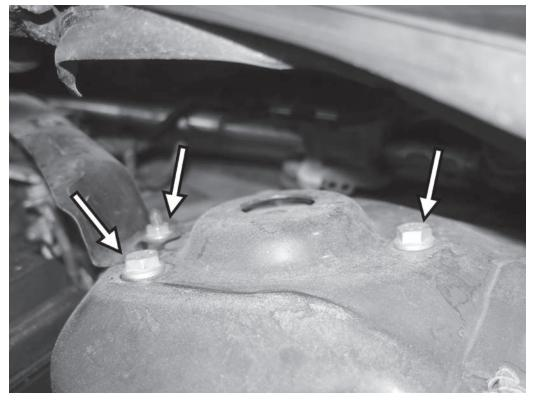
9) Lift up the rain tray under the hood. Then, holding the strut assembly from falling, remove the three nuts holding the strut assembly and remove it from the car.
