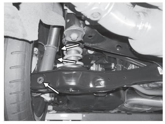
27) With the suspension still in this position, adjust the overall length of the shock. Turn both the lower body of the shock and the lock collar up on the threaded body until the bottom shock bolt hole lines up with the hole for the shock in the lower control arm. The shock bolt should be able to easily be installed or uninstalled through the lower control arm and the shock hole.
