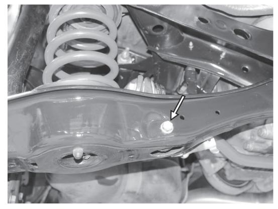
15) Disconnect the rear sway bar from the lower control arm on both sides of the car.
