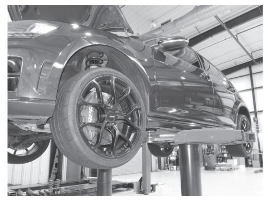
1) Place the vehicle on a lift or secure jackstands, and remove all four wheels.
