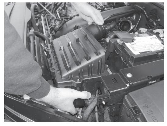
7) Firmly grab underneath the left side of the airbox and under the airbox outlet, and pull directly up on the airbox to separate it from the three posts it is sitting on. Lift the airbox about one inch (25mm).
