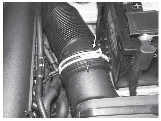
5) Squeeze the clamp on the accordian hose on the back of the factory airbox, sliding it back and off the connection to the airbox. Separate and remove the accordian tube from the airbox.
