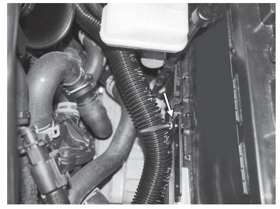
11) Pull the secondary air hose back so that the installed filter sits under the outlet of the APR airbox. Once the filter is out of the way, tighten the cable tie around the hose and secure the hose to the bracket previously installed on the side of the battery tray.
