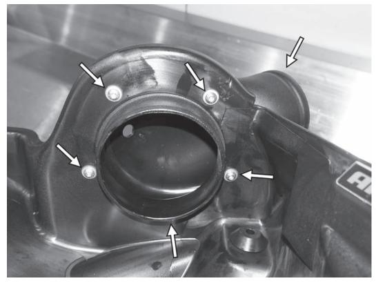
3) Install the airbox outlet pipe to the side of the APR airbox. Make sure the outlet pipe is oriented correctly before securing it with the five shorter 3mm allen screws and rubber washers. Tighten the five screws to 28 in-lbs (3.1 Nm).
