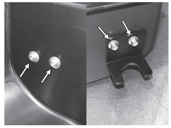
1) The APR airbox assembly must first be built. Begin by attaching the included bracket to the side of the APR airbox with the two holes. Install the two longer 3mm allen screws from the inside of the airbox with a rubber washer. Then install the bracket as shown and secure the bracket with two more rubber washers and the two 8mm nuts. Tighten the two screws while holding the nuts to 28 in-lbs (3.1 Nm).
