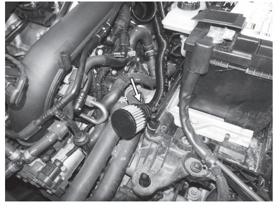
9) If equipped, install the supplied secondary air filter (sold separately) onto the end of the secondary air hose that was attached to the back of the factory airbox. The filter simply snaps onto the connection of the hose. Tuck the filter and hose down and out of the way, and secure with the supplied cable tie.
