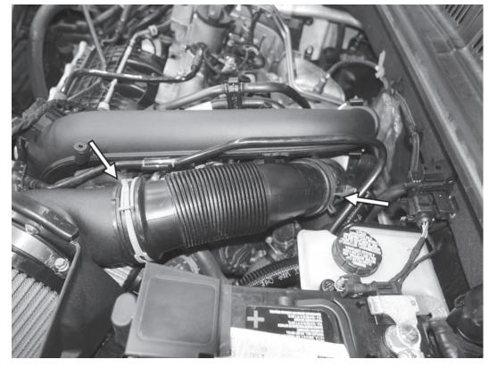
13) Install the accordian tube, connecting it to the APR airbox outlet and to the inlet of the turbo. Squeeze each of the spring clamps and slide them into their original positions to secure the accordian tube to the engine. If your accordian tube uses screw clamps, tighten them to 4Nm (35 in-lbs).
