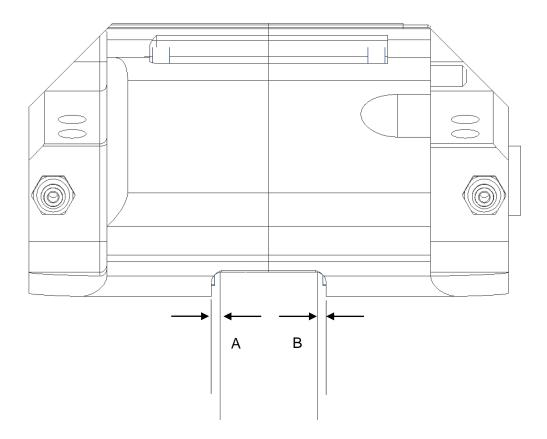
**NOTE:** For vehicles with splash plates mounted behind the hub: If you have completely removed your vehicle's splash plates, it will affect the caliper centering since the hub has now moved inboard. It would be preferable to cut the center of the splash plate out and reinsert it behind the hub to get the centering correct.
