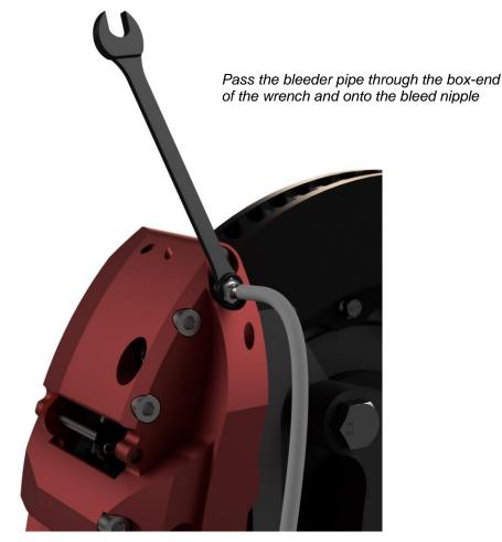
• Use a brake fluid that is compatible with the seals in your brake system. DINAN recommends Glycol based brake fluids that meet DOT 4 specifications or higher. Do not use Silicone based brake fluids with DINAN calipers. For recommendations on specialised high-temperature or competition brake fluids, please contact DINAN.
