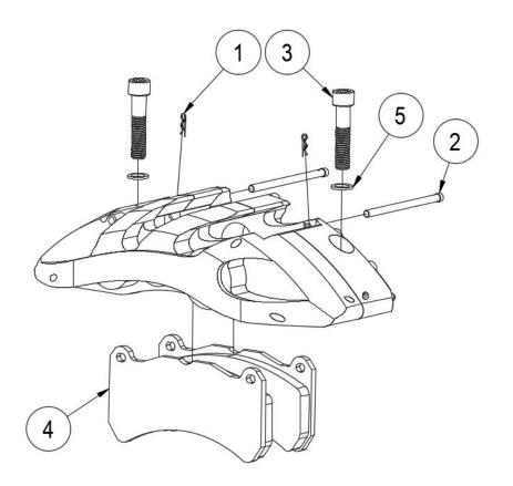
The international standard width for the pads used in the S6L caliper is 164.50mm. If the replacement pads you are fitting is wider than 164.50mm the edges need to be filed to fit.
