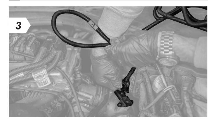
• Now connect the end of the tuning module wiring harness marked "A" to the disconnected connector and the other end to the sensor.
