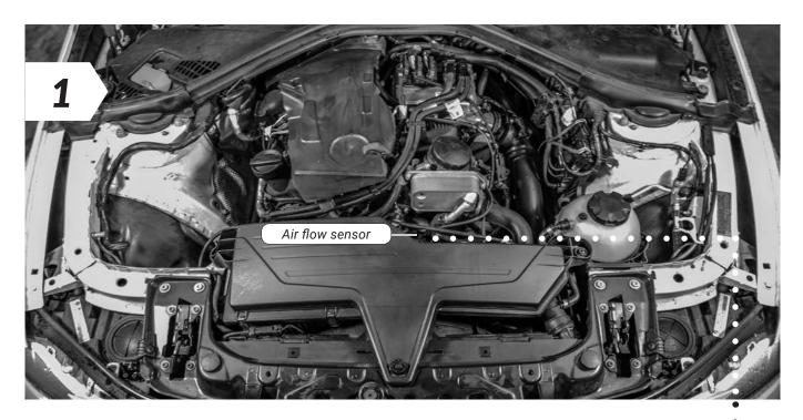
First locate the air flow sensor connection in your engine bay.
