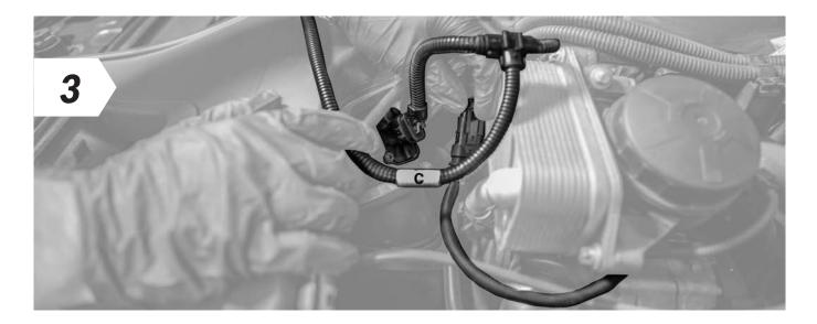
• Now connect the end of the tuning module wiring harness marked "**C**" to the disconnected connector and the other end to the sensor.
