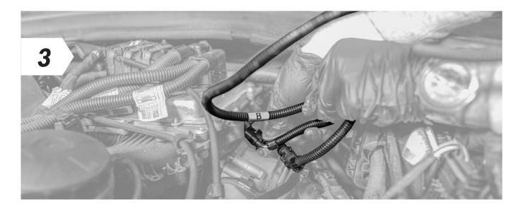
• Now connect the end of the Dinan wiring harness marked "**B**" to the disconnected connector and the other end to the sensor.
