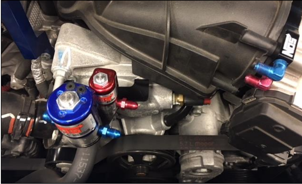
Figure 12 – Solenoid Bracket Mounted Location
