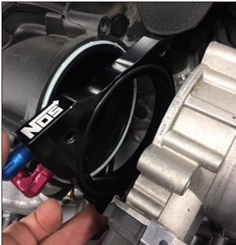
Figure 6 – Nitrous Plate Installation
