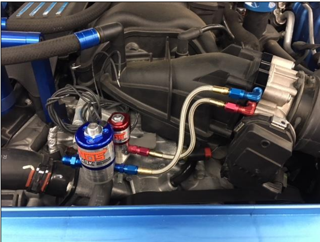
Figure 13 – Installed Nitrous Solenoids
