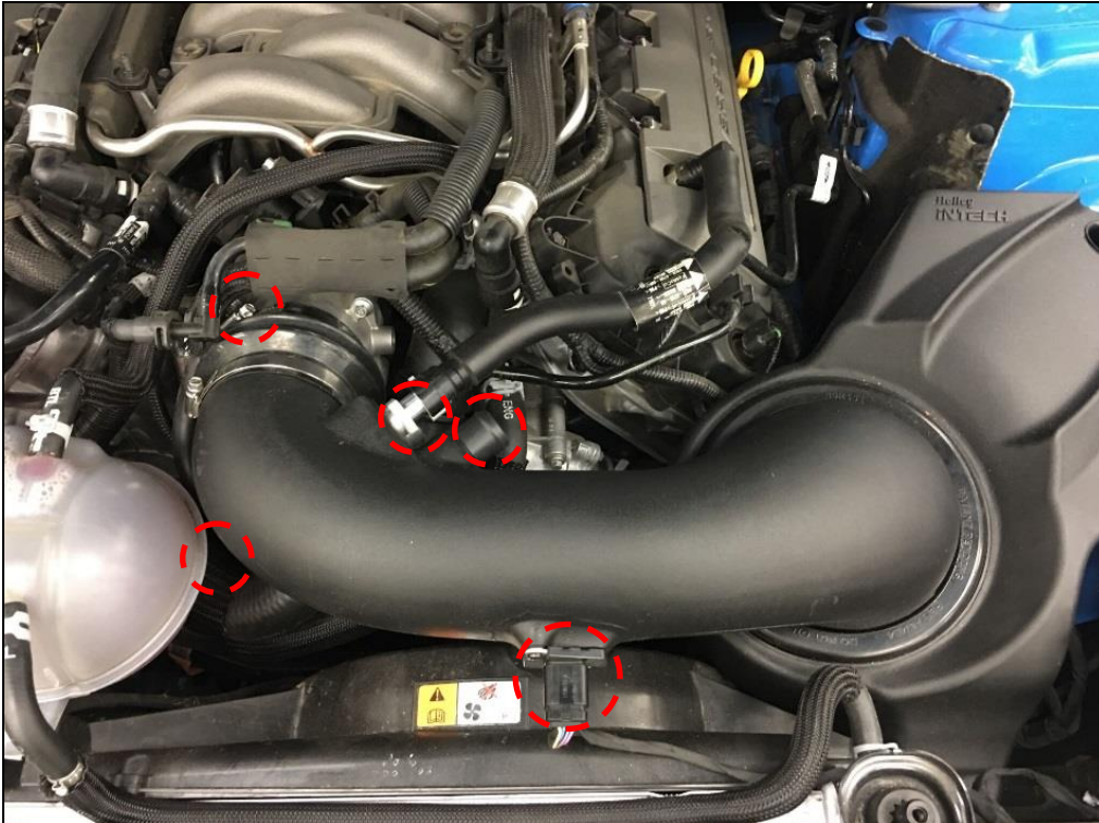
Figure 7 – Intake Air Tube Removal (Holley® Intech Shown, but Factory Intake is Similar)
