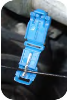
Figure 3 (T-Tap connector installation)
