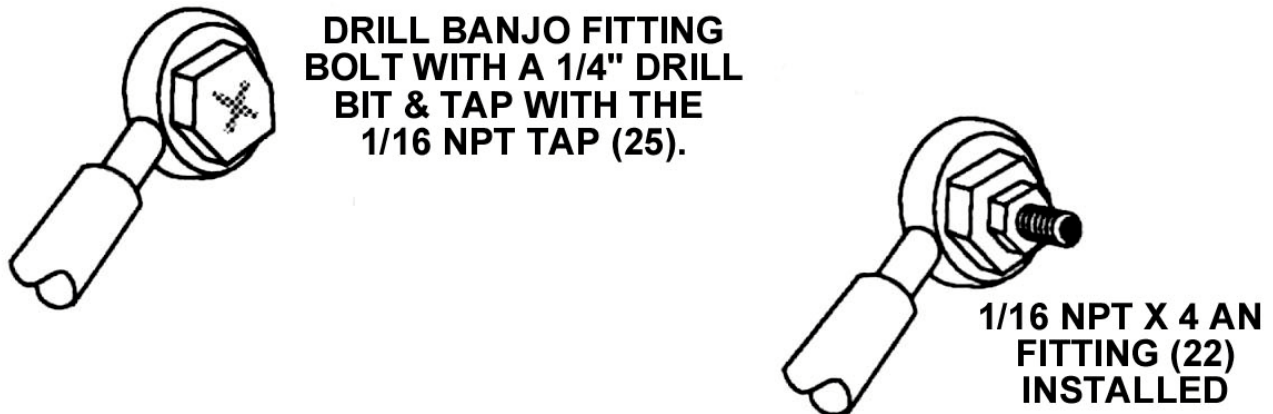
Figure 8 Schematic of "Drilled Out" Banjo Fitting
