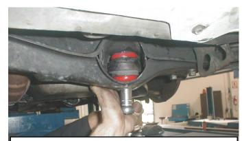
Grease inside of subframe where the bushing contacts metal. Reinstall in reverse order and tighten all fasteners to factory torque. Always use new cotter pins.
