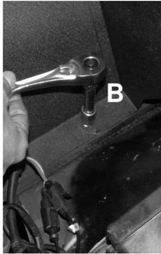
A&B) Tighten and secure heat shield using the 10mm socket and ratchet.
